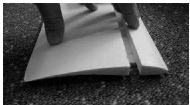
Foam core cut to accept spar
