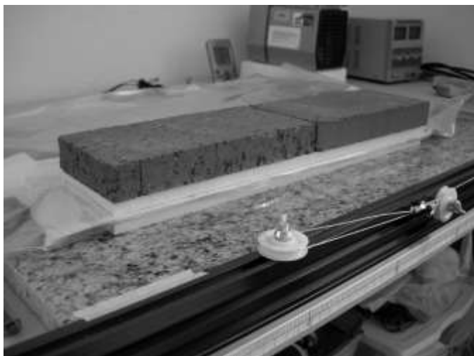
Assembly inside vacuum bag under weights. Wire cutting guide pulleys on bench in foreground
