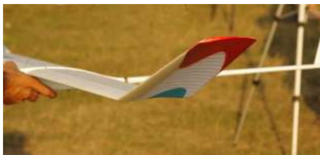
F1A of Amit Kidron ISR (2.). All four F1A in the second fly-off had LDA airfoils!
