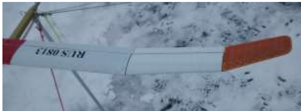
General view of wings – carbon structure but finished in white, geodetic bracing between the leading edge and the spar.
