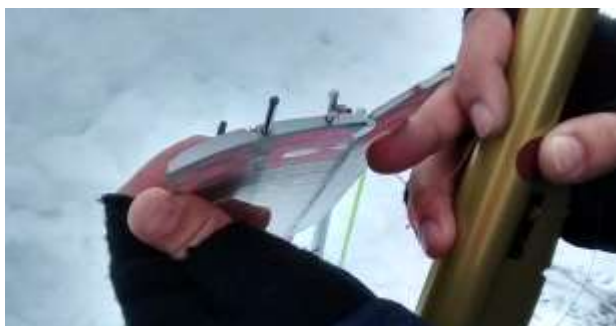
Root wing section with flap raised
