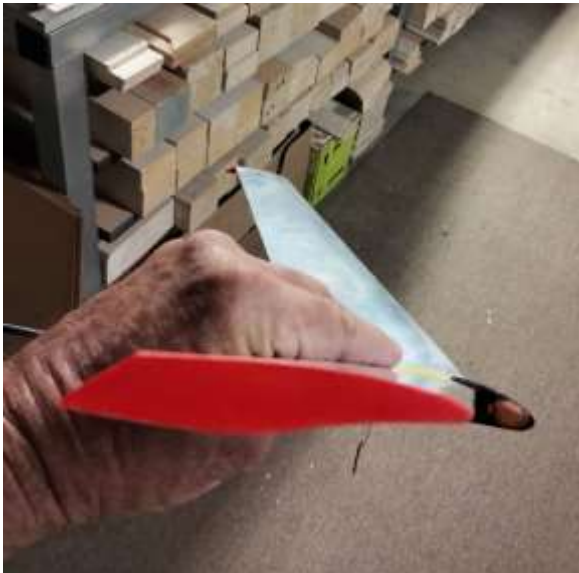
Modified Michael Towell winglets to allow a clean release with thumb under the wing
